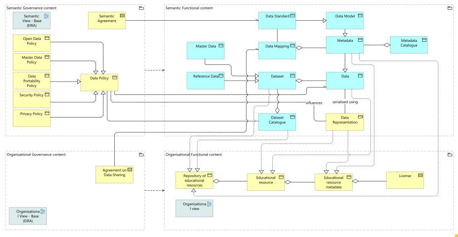
Figure 24 - Use case 4 reference architecture semantic view.
